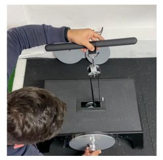
Stand on unit with both feet. Press belt release/adjustment pin to bring handle/accessory to desired height. Release pin.
